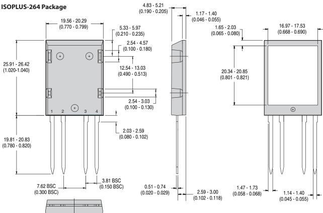
NOTE: Bottom heat sink meets 2500V<sub>rms</sub> isolation to the pins.
